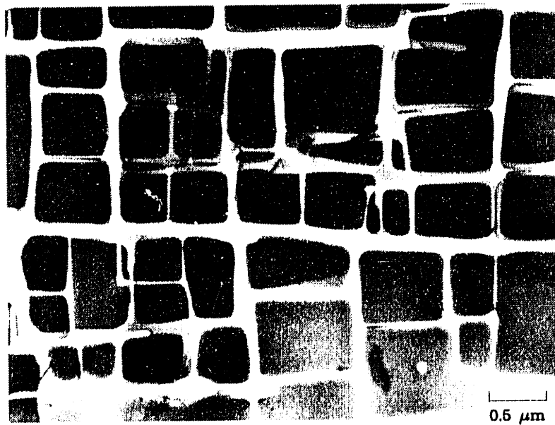
Figure 1-3: TEM micrograph of undeformed CMSX4 – \langle 001 \rangle direction out of the plane
