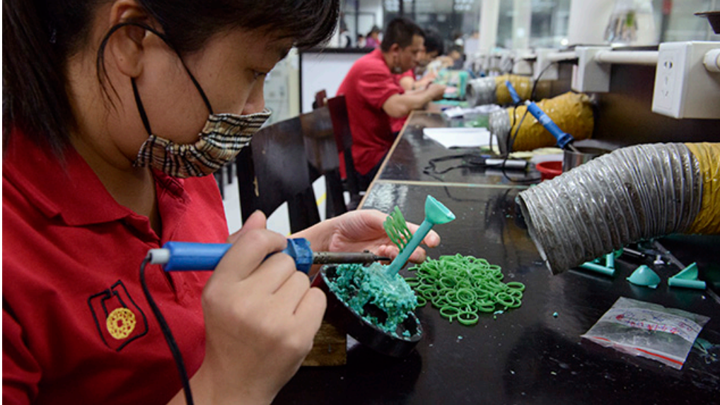
Figure 6: Specialized factory in Guangdong producing wax molds for rings (photo by Eric Welch courtesy of Chow Tai Fook, Hsu et al. 2014)
