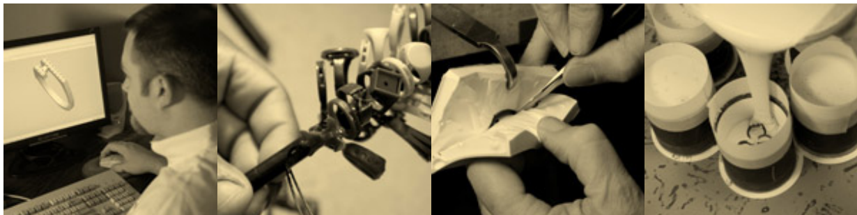
Figure 5: Jewelry production stages at Flexible SME Producer Au Enterprises: CAD modelling, preparing a set of 3D printed rings for casting, pouring wax into a mold, and taking a finished ring from the mold
