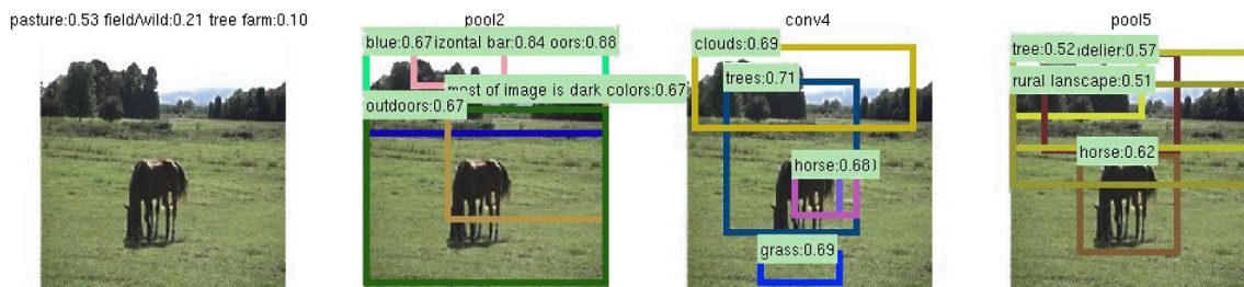
Figure 4-13: Interpretation of a picture by different layers of the Places-CNN using the tags provided by AMT workers. The first shows the final layer output of Places-CNN. The other three show detection results along with the confidence based on the units' activation and the semantic tags.
