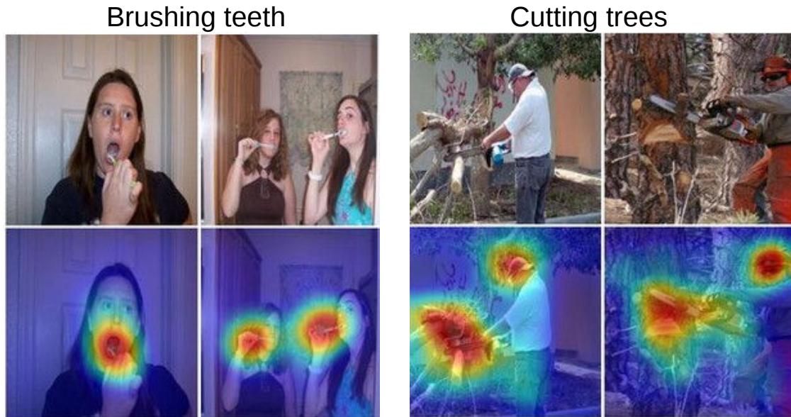
Figure 6-1: A simple modification of the global average pooling layer combined with our class activation mapping (CAM) technique allows the classification-trained CNN to both classify the image and localize class-specific image regions in a single forward-pass e.g., the toothbrush for brushing teeth and the chainsaw for cutting trees . It produces a visual explanation for the decision made by the CNN.
