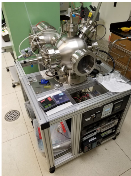
Figure 3-7: In house built thermal evaporator for pentacene deposition.
