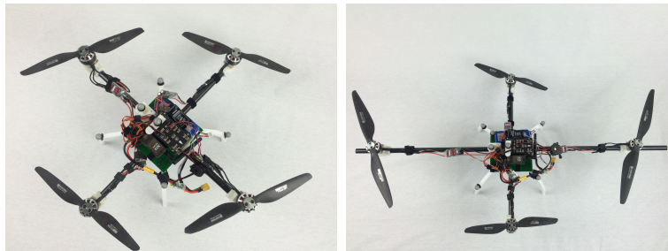
Figure 8-20: Optimizing a quadcopter with flight time metric and geometry constraints. Left: a standard quadcopter. Right: optimized rectangular quadcopter.
