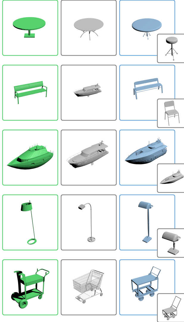
Figure 4-14: Comparison of retrieval with mean shapes only and manifold representation for the Light Field descriptor. From left to right: query shape (green), closest mean shape retrieved (gray), closest parametric shape retrieved with parameter fitting (blue) with its corresponding mean shape (gray). We observe that using the parametric shapes we retrieve models that are more similar in geometry but may lie on a different class.
