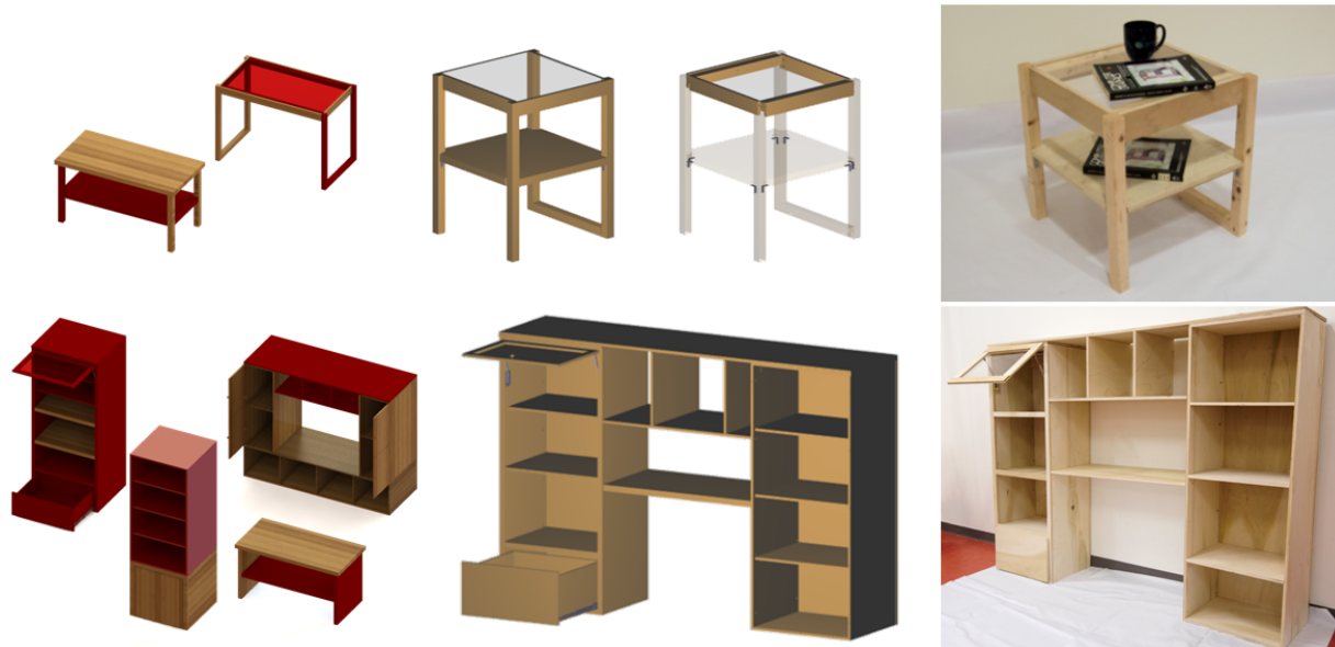
Figure 5-9: From left to right: input designs, models created using the system, and fabricated results. We highlight the connecting elements on the first model by making all principal elements semi-transparent.
