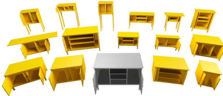
Figure 1-3: An example of a parametric design. The original design is shown in gray, and the new designs generated by varying the parameters are shown in yellow.
