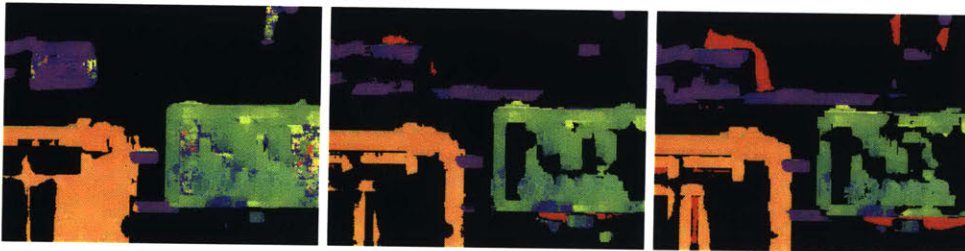
Figure 3-6: Depth Maps from using other criterias. From left, noise criteria used are Standard Deviation, SNR, Kurtosis. Calibration and resolution is different.
