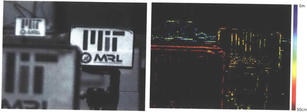
Figure 3-9: Resulting Depth Map of applying Heisenberg Depth Uncertainty. Depth scale has been reduced to 6m so it is easier to compare the different objects visually.
