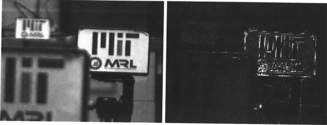
Figure 2-3: Example of Focus Measure operator for object at 2m distance. We have used Variance of Wavelet Coefficients.
