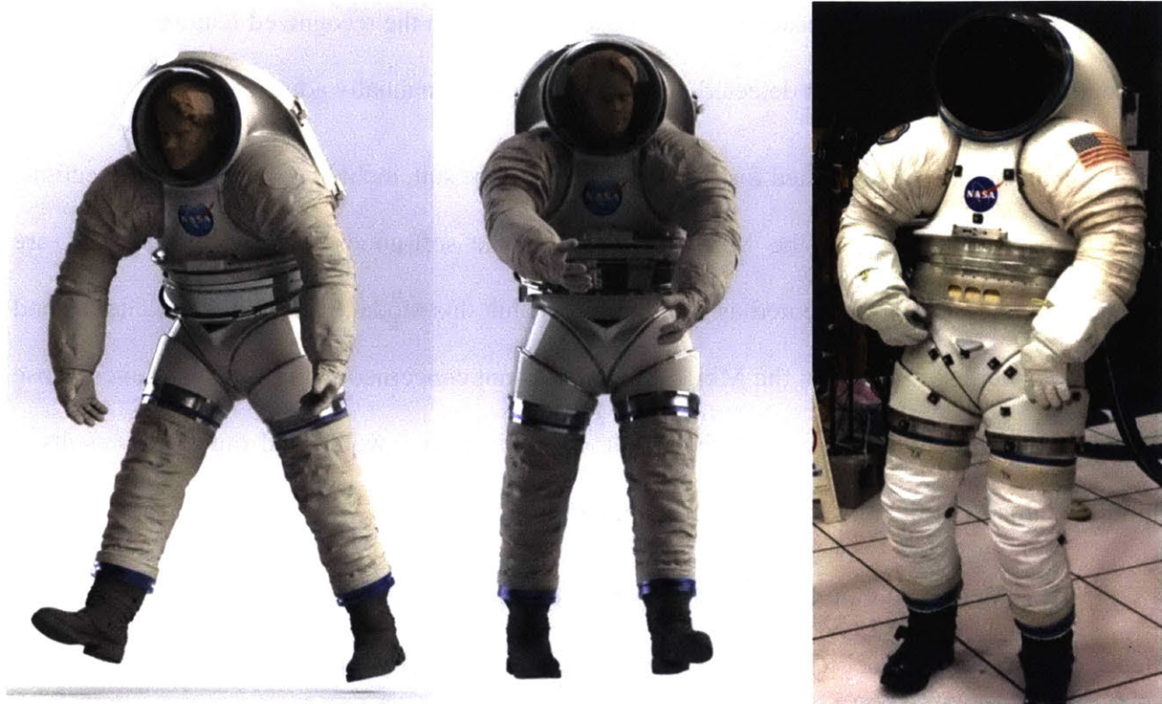
Figure 2: The Mark III (MkIII) Space Suit Assembly (SSA) Rigid-Body SolidWorks Model (Left and Center). The MkII SSA (Right).
