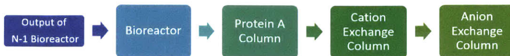
Figure 3-5: Simplified flowsheet of the antibody production process. The bioreactor size was 2000L and was operated in the fed-batch mode. The column loadings were typical of an antibody purification process [231].
