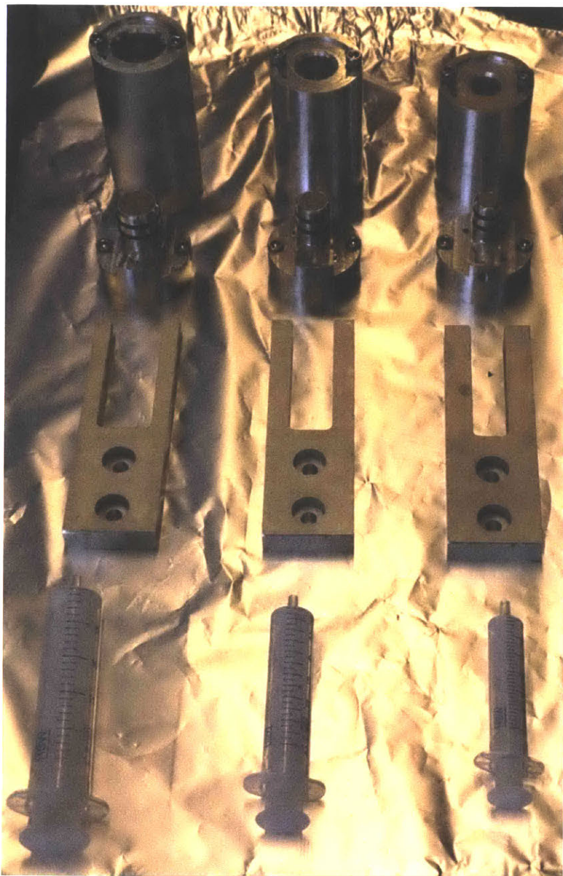
Figure A2.16: Photograph showing resin vessel inlets, resin vessel bodies, and forks for three scales with the syringes they accommodate. On the left is the 24mL scale, the 12mL scale is center, and the 6mL scale is on the right.
