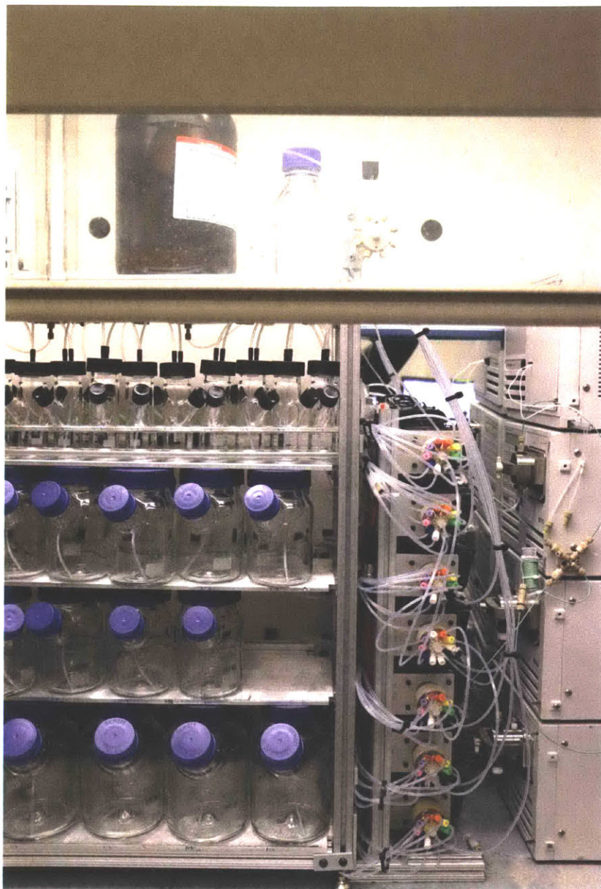
Figure A2.14: Photograph of the plumbed valves. The union cross, check valves, and static mixer on the high pressure side are also visible.
