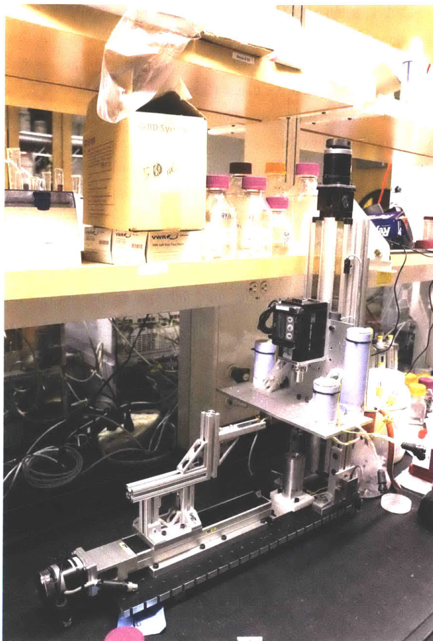
Figure A2.15: Photograph of the reactor module prior to plumbing and wiring. The fork is mounted to the horizontal actuator, but is not in its final configuration (see CAD drawings). The 6mL resin vessel body and universal outlet are clearly visible on their mounts, and the 6mL inlet is just barely visible under the middle plate. Three activation reactors, the column changing valve, and both pressure sensors are also clearly visible. The yellow wires are thermocouple leads and the white wires are cartridge heater leads. The grey wires are leads for pressure sensors, motors, and the limit switches used to home the motors.
