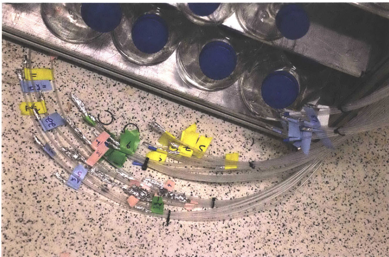
Figure A2.10: Liquid lines were bundled by valve and labeled. If the labels fall off it is difficult to trace them later. Foil caps prevented dust from entering prior to connecting the valves.
