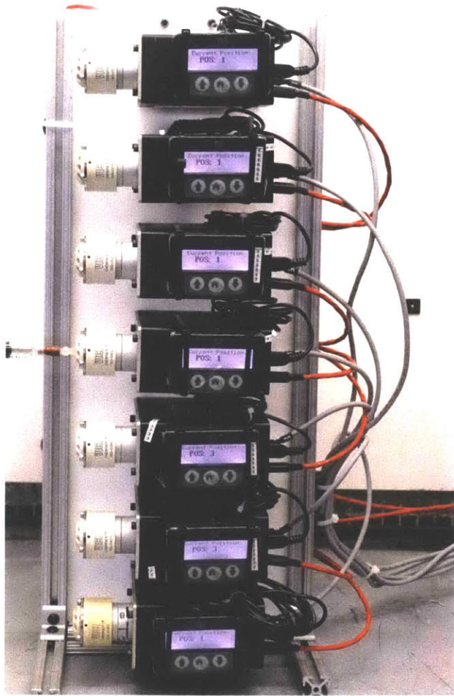
Figure A2.12: Side view of the valve module. Manual controllers were affixed to each valve to facilitate troubleshooting and system verification.
