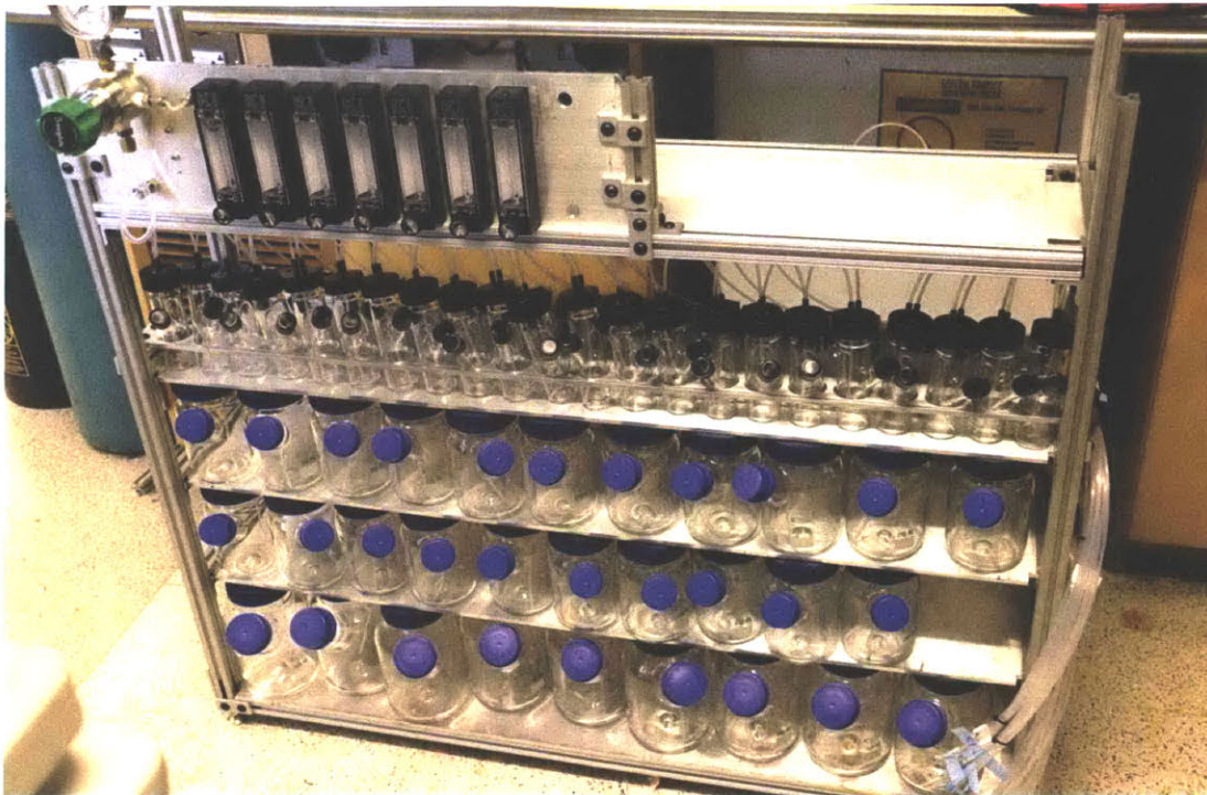
Figure A2.8: Front view of the assembled shelf module with bottles, prior to installation of the engraved labels.
