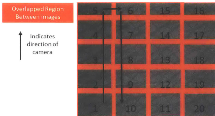
Figure 7: Camera Motion during Experimentation: The head of the Quick Vision Active system moves along the direction of the arrows towards increasing number of image frames, as indicated in the figure. The thick red borders indicate the amount of overlap between the frames. There are 20 images acquired in a 1 in 2 area on the skin.
