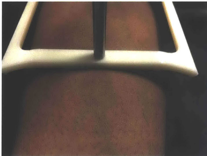
Figure 35: Contoured Base along the ROI: This base helps increase device stability during experimentation
