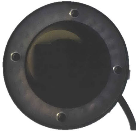
Figure 31: Ring Light Flush with Camera Lens for a Convenient Form Factor and Maximum Portability
