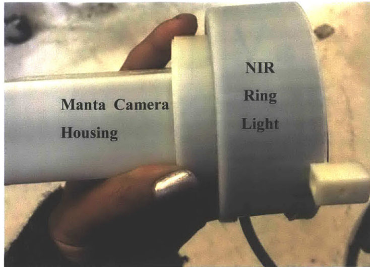
Figure 32: Camera and Light Fixture: By keeping the light hidden from view, we keep a small form factor to make it handheld and more aesthetically pleasing.
