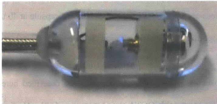
Fig. 4. Capsule design for low numerical aperture imaging. Motor rotates a prism only (no lens carriage) and the working distance of the focusing optics is long.
