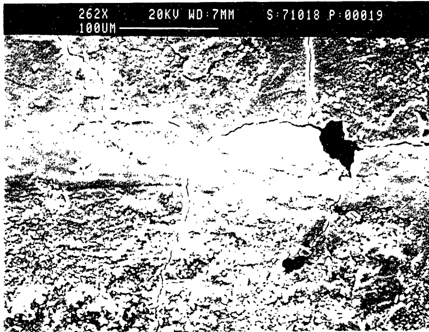
Figure 7-33: Mortar in the vicinity of the epoxy crack tip (midheight, epoxy was at the top)
