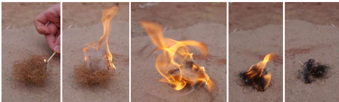
Figure 35: Selected Frames from Coconut Fiber Mattress Ignition; left to right: 0 sec., 2 sec., 4 sec., 9 sec., 18 sec.
