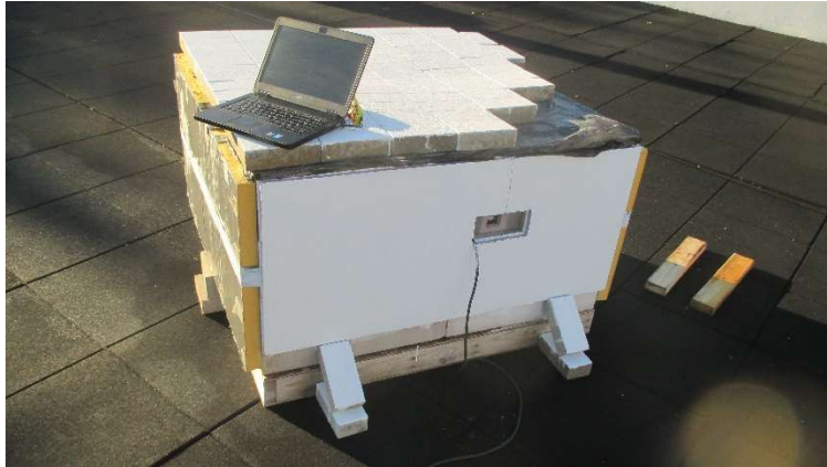
Figure 15: Test 4 with North and South foil-faced exterior insulation and East and West white-painted exterior insulation
