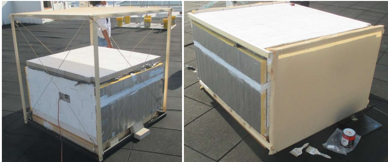
Figure 12: Test 3 experimental setup with shade nets installed
