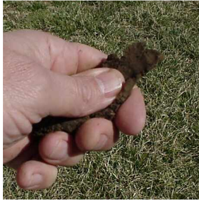
Figure 13. Soil moisture feel test
