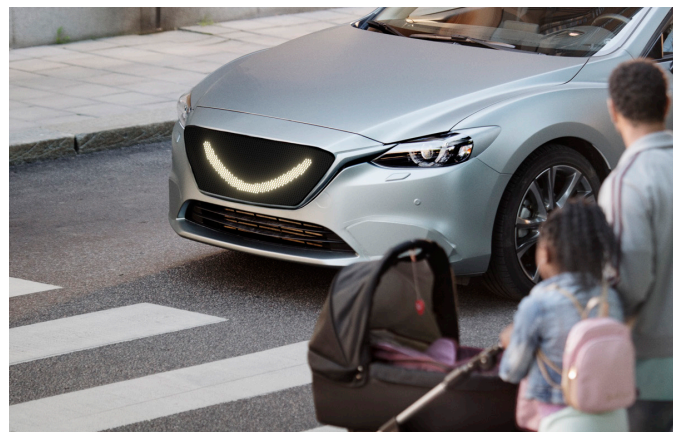
Figure 2.4 & 2.5: current devices used by drive.ai (left) and Semcon (right) for vehicle-pedestrian communication. Left image from www.drive.ai . Right image from https://semcon.com/ .
