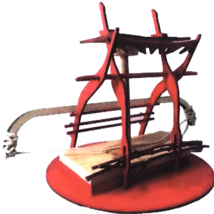
Figure 37 Fire-drilling Machine: Hold the structure with one hand on the top to stable it while floating on the water. The other hand pushes the bow drill forward and backwards. The wood stick would spin on the wood base and could possibly start a fire if operated skillfully.
