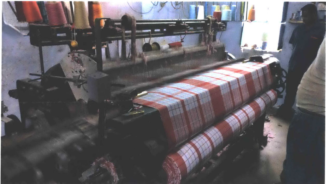
Figure 22: A retro-fitted rapier loom in operation
