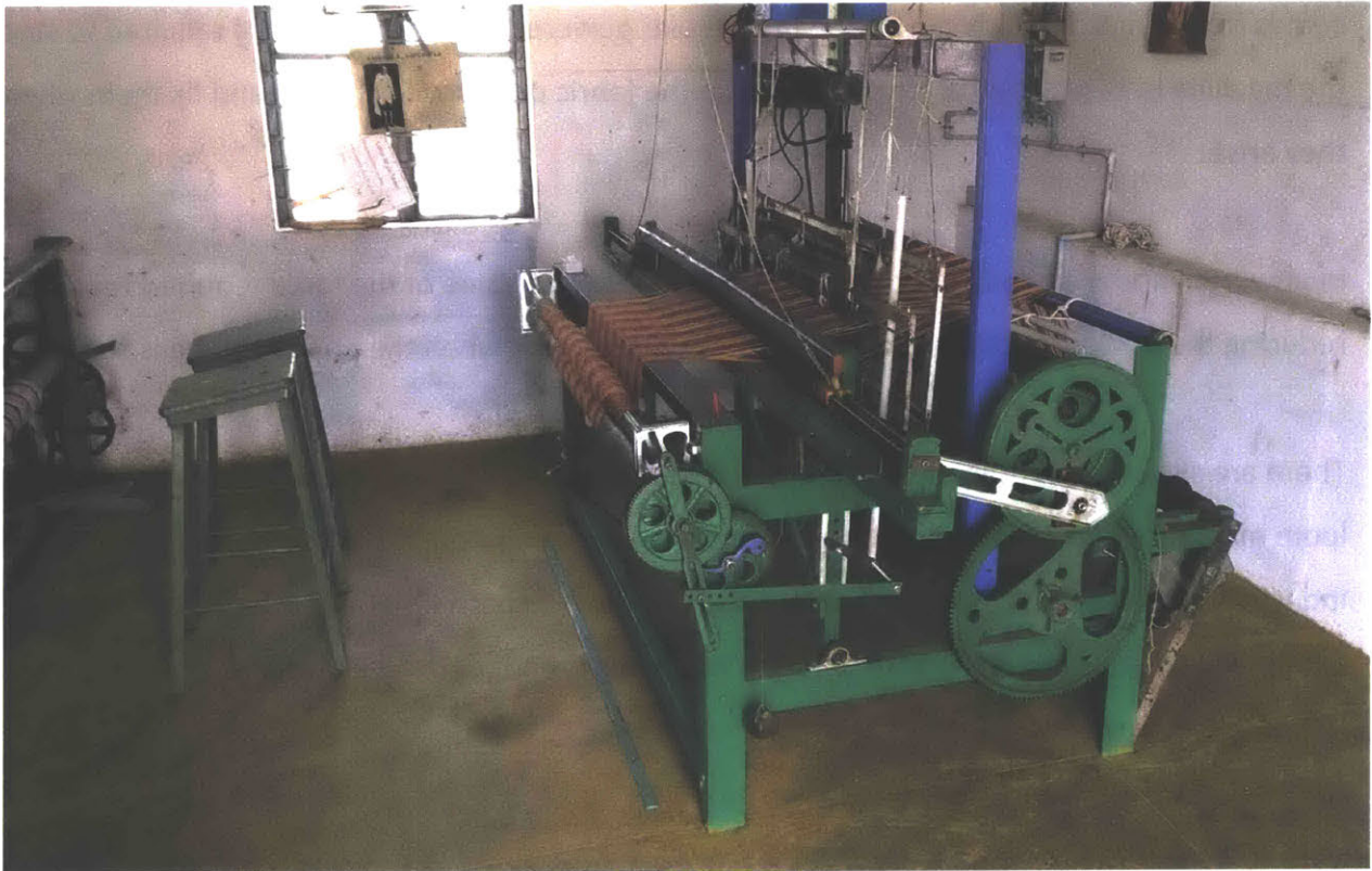
Figure 8: Sun Kharga, NRG Solutions' Energy Efficient Loom
