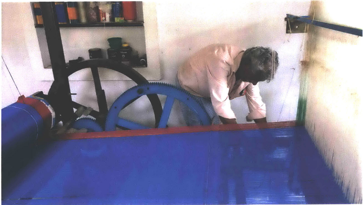
Figure 21: The flywheel and gears on the loom visible next to its inventor
