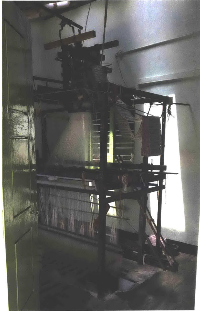
Figure 6: A Jacquard loom in the weaving village of Negamam, Tamil Nadu. Note the shedding mechanism atop the loom with punch cards.
