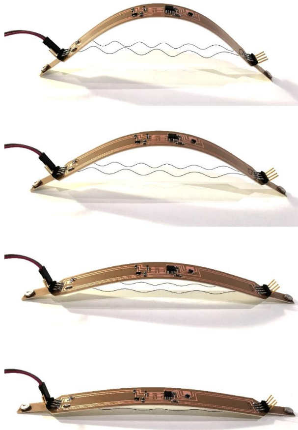
Figure 25: SMA Actuator providing controllable curvature
