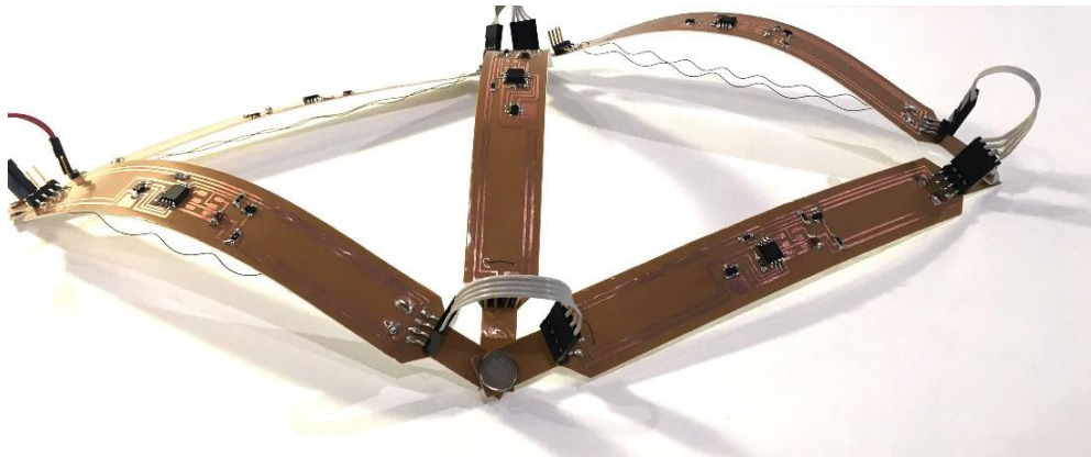
Figure 26: SMA Actuator creating variable curvature
