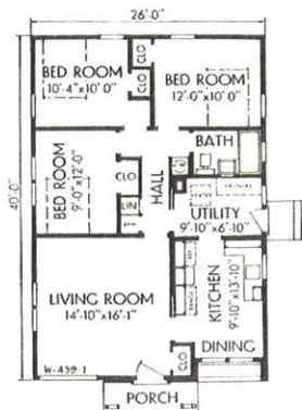
Plan 1, with Utility Room, No Basement
