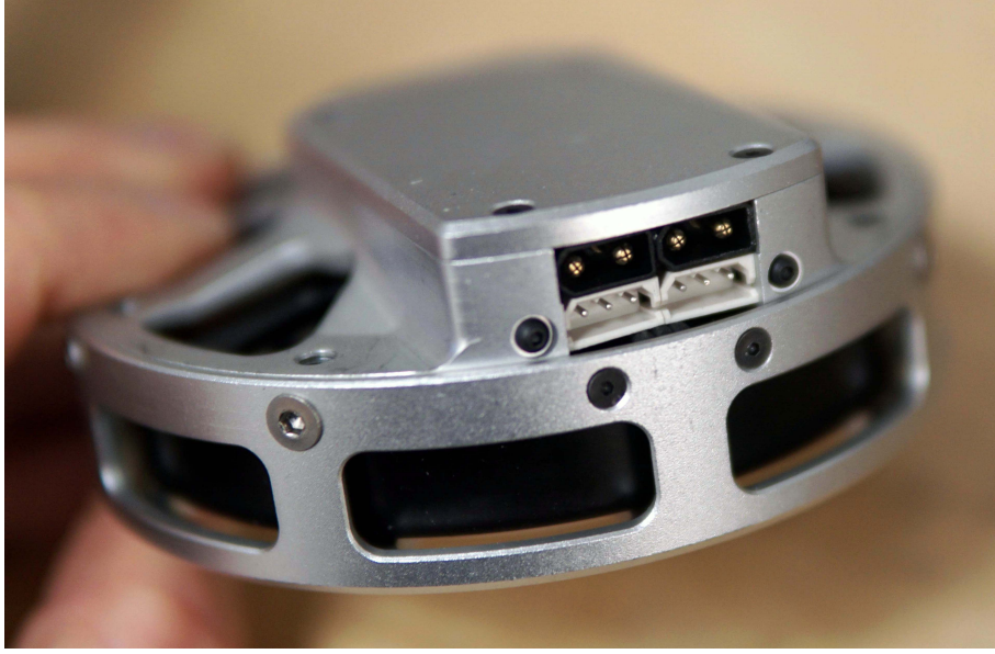
Figure 2-13: View of the connectors to the actuator. Two XT-30 connectors are used for DC input power, and two 3-Pin Molex SPOX connectors are used for CAN. Each pair of connectors is in parallel, so actuator modules can be easily daisy-chained.
