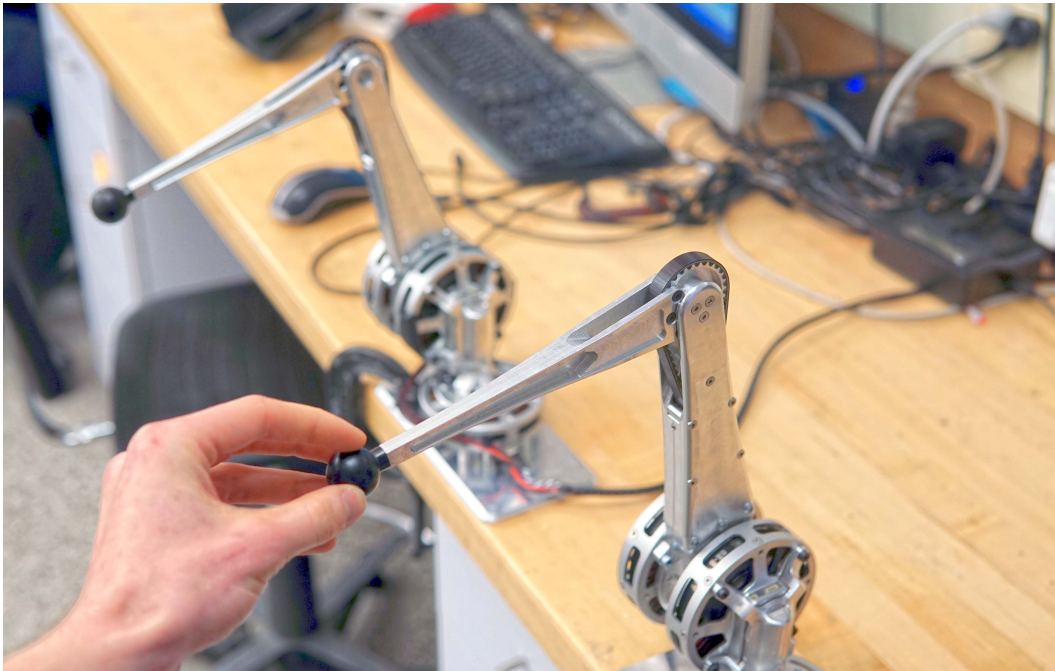
Figure 4-1: Teleoperation and haptics setup consisting of two 3-DOF arms, with feet replaced by smooth spheres.
