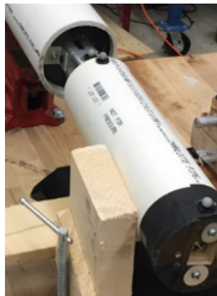
Figure 3-8: Vicon Pearl Placement for \theta_A Measurement on Artifact
