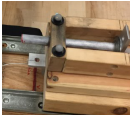
Figure 3-6: Vicon Pearl Placement for V_I Measurement on Impactor
