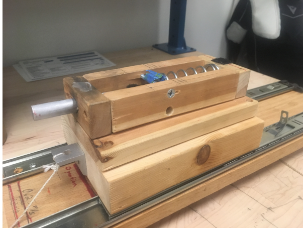
Figure 3-2: Impactor Design for Experimental Benchtop Rig
