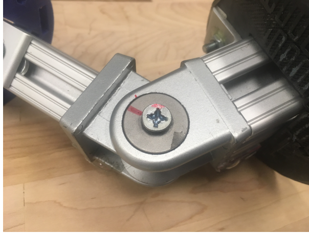
Figure 3-5: Artifact Pin Joint for Enabling Restricted or Free Rotational Motion
