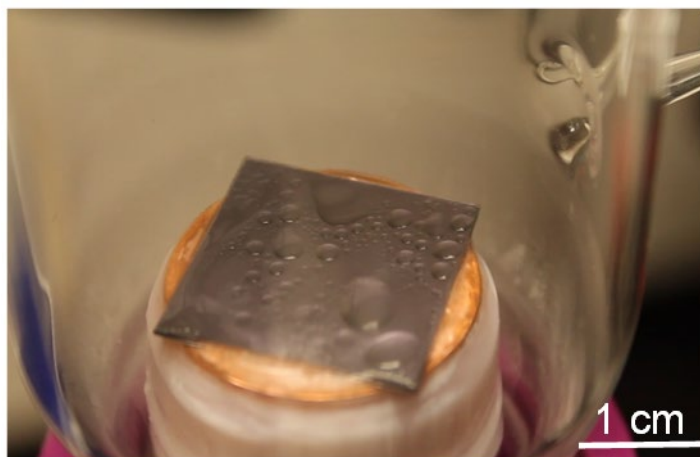
Figure 23. Dropwise condensation of butane on 6F-IPA infused SiO 2 micro-pillared surface.
