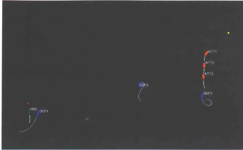
Figure 4-6: Defensive Formation Adapts Autonomously to Threat. Vehicles orient based on opposing formation and take station in a trail position, a picket position, and a screening position. Determining and moving to positions requires no inter-vehicle agreements.
