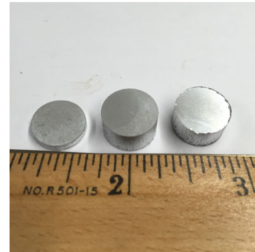
Figure 5.13: The finished pellets are about 0.5" wide and 0.25" high. The pellets are much easier to handle than the loose powders, especially during the arc melting step.
