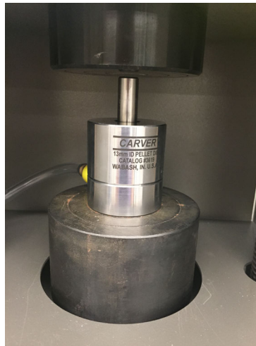
Figure 4.7: A Carver™ 13mm ID pellet die was used for niobium cold working. The stage applies force to the die's pushing rod and core die .
