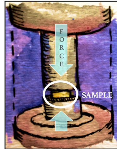
Figure 4.8: A schematic showing the interior of the die. The Nb samples were centered in the inner faces of the interior steel pushing rod (top) and core die (bottom).
