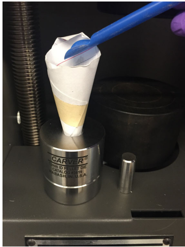
Figure 5.11: Ni/Al powder mixture is transferred to the pellet press die using a funnel and a disposable scoop
