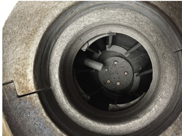
Figure 5.15: The five buttons made in the arc melter were heat treated in a high-temperature graphite furnace under an inert environment for 24h at 1200°C. The photograph shows the buttons arranged in the furnace prior to beginning the heat treatment. The purpose of the heat treatment was to grow large grains, so that the TGS measurements could be easily carried out within the boundaries of a single grain if the buttons were used for measurements. The furnace pictured here is in the Allinore lab at MIT.
