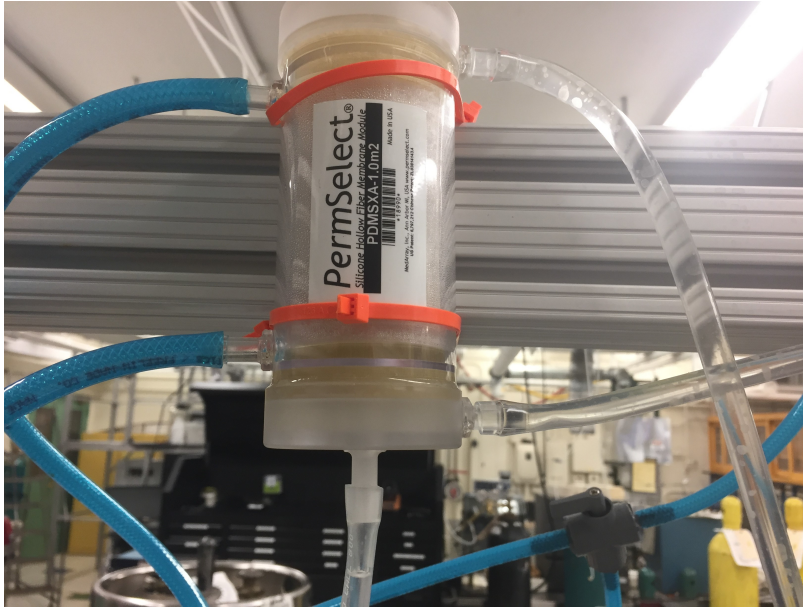
Figure 2-6: PermSelect degassing system. Connections on the right side are flow inlet and outlet, connections on the left are vacuum ports.
