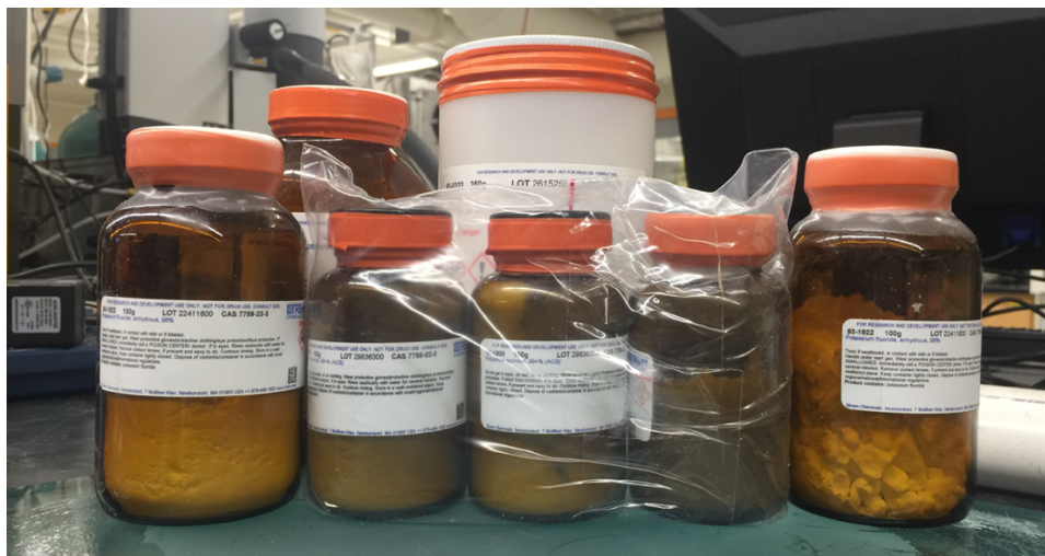
Figure 8 Alkali-halide salts chosen for irradiation include NaCl, NaI, NaF, NaBr, and CsF for their distinct f-center behavior and potential applications to IF2D.
