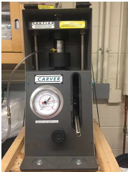
Figure 10 The CARVER Pellet Press has a 20,000 lb pressure limitation. In this case, a 13 mm pellet die was used that has a pressure limitation of 18,000 lb. This setup includes a vacuum pump to remove any atmospheric effects on the salt being pressed.
