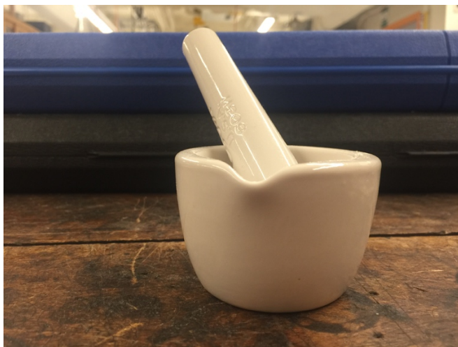
Figure 11 Mortar and pestle used to grind the salts into a fine powder similar to confectionary sugar.
