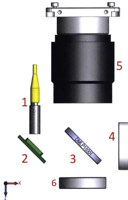
Figure 2-6: NODÉ Components that require alignment for system functionality. Components indicated are 1: Collimator, 2: FSM, 3: Dichroic, 4: Mirror, 5: Beacon Camera, and 6: Filter. Required alignment of each optic is listed in Table 2.3
