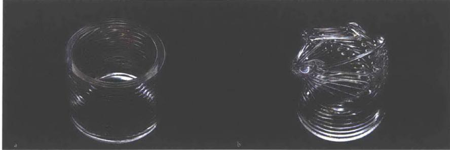
*Figure 3-22:* (a) cylindrical tool path under standard print conditions and (b) identical tool path showing adhesion errors and bridging instability phenomenon
