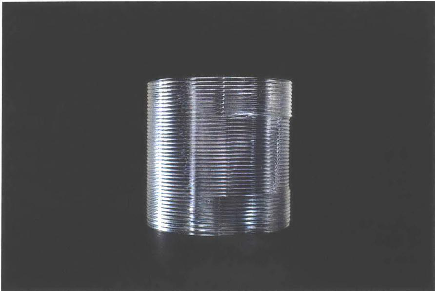
*Figure 3-12:* feed rate experiment with half of each layer in the test section printed at double the control feed rate (20 mm/s)
