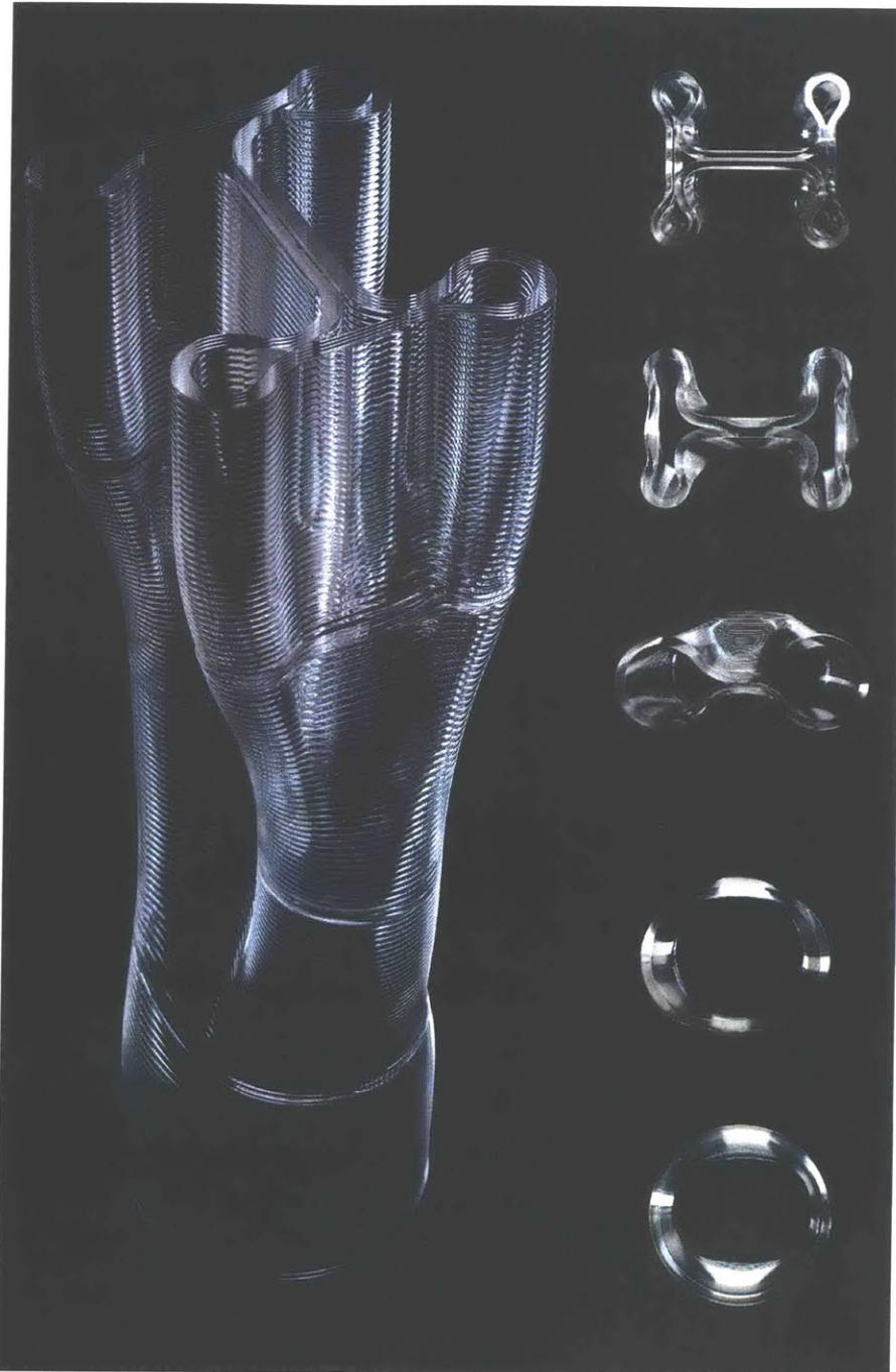
Figure 4-6: 4 component fluidic structure with morphing sectional topology with sections at joints and ends shown right 75
