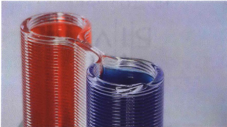
*Figure 4-1: 3D printed glass vessel, with colored liquid illustrating multiple channels*
