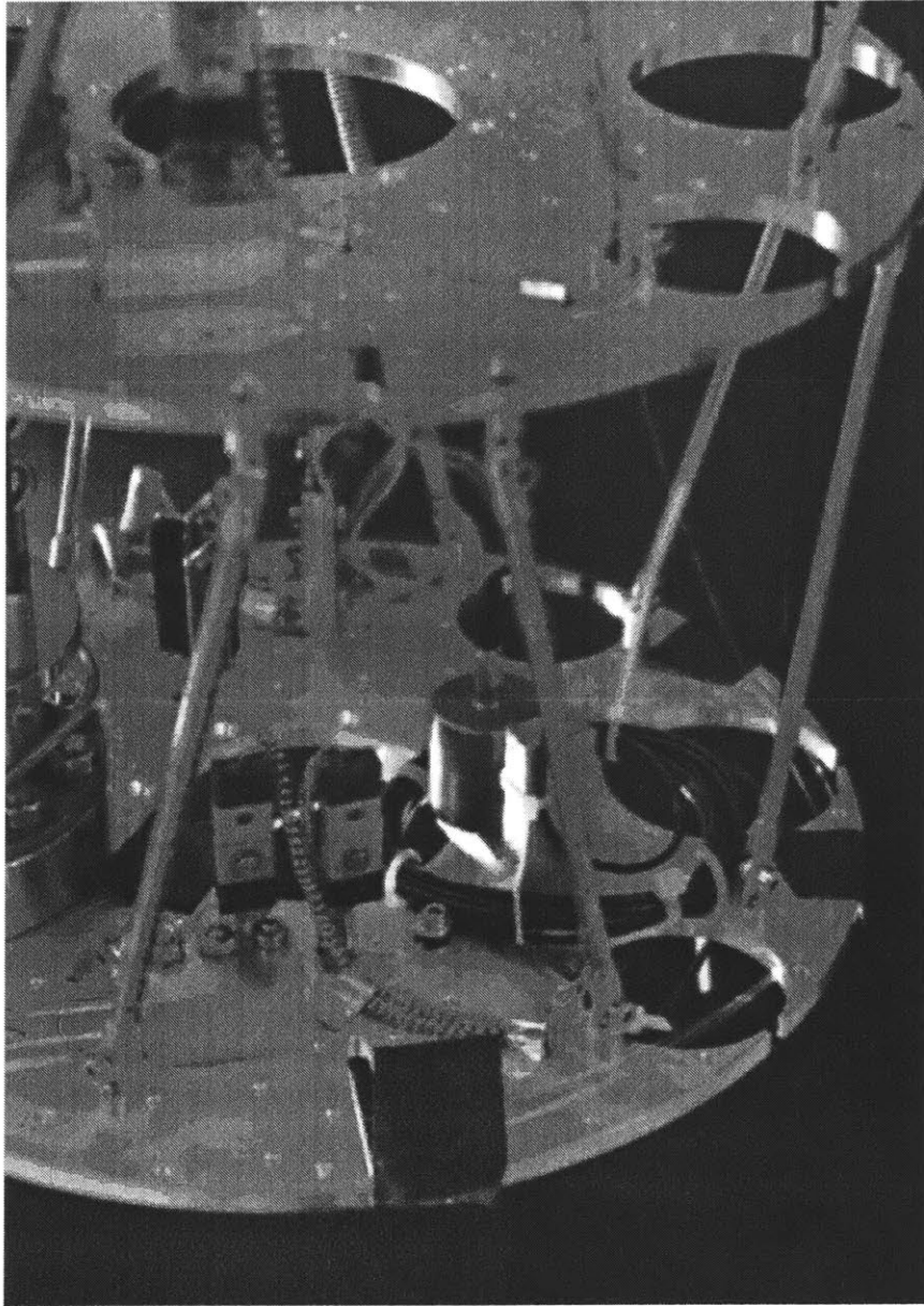
Figure 2-11: Mounting setup of the accelerometer as mounted on the Mixing Chamber plate on Olaf. One of the main concerns when running the blue readout cable came in the form of peizo-capasitances created when the readout cables are mechanically stressed. These capacitances could induce additional noise in our readout signal, which is why you see zipties and fishing lines (not pictured) to tie down these cables to the various support beams
