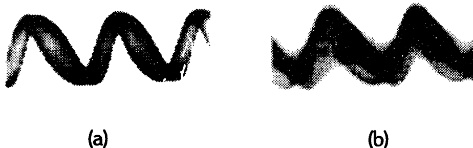
Figure 4.40 Beat note between SBS lasers with a small frequency bias (a) with light dither, and (b) with misadjusted dither. Cavity H.
