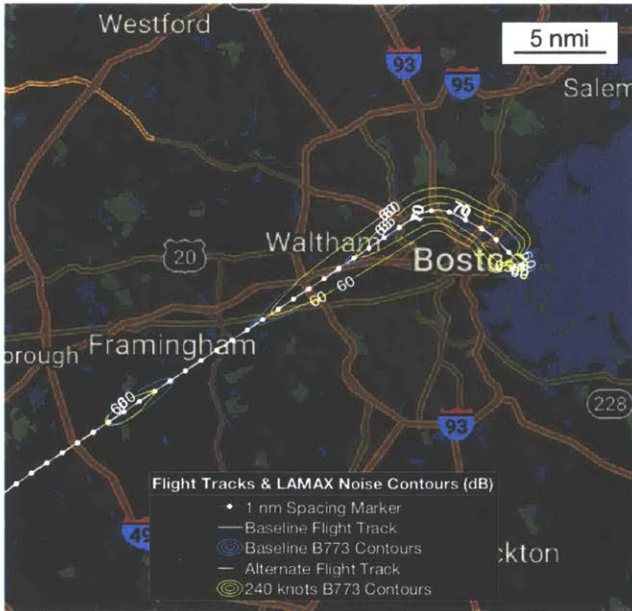
Figure 98. Noise exposure reduction for the Boeing 777-300 departing runway 33L via the BLZZR4 departure on a standard climb profile compared to a 240-knot reduced speed departure. Noise Model: NASA ANOPP
