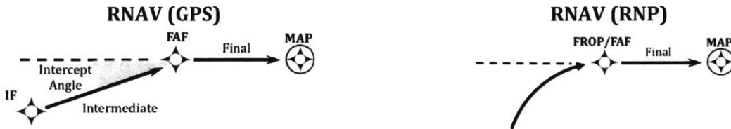
Figure 35. Intermediate and final approach geometry for RNAV and RNP procedures
