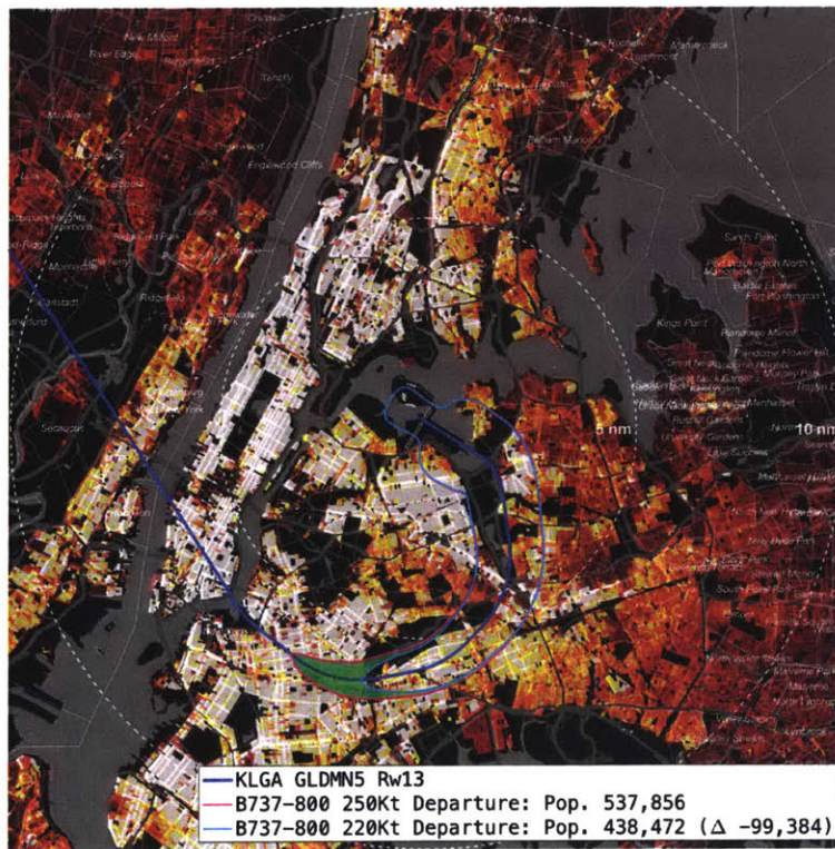
Figure 85. B737-800 noise benefits from a reduced-speed departure on the GLDMN Five RNAV SID from LGA runway 13 (60dB L MAX )
