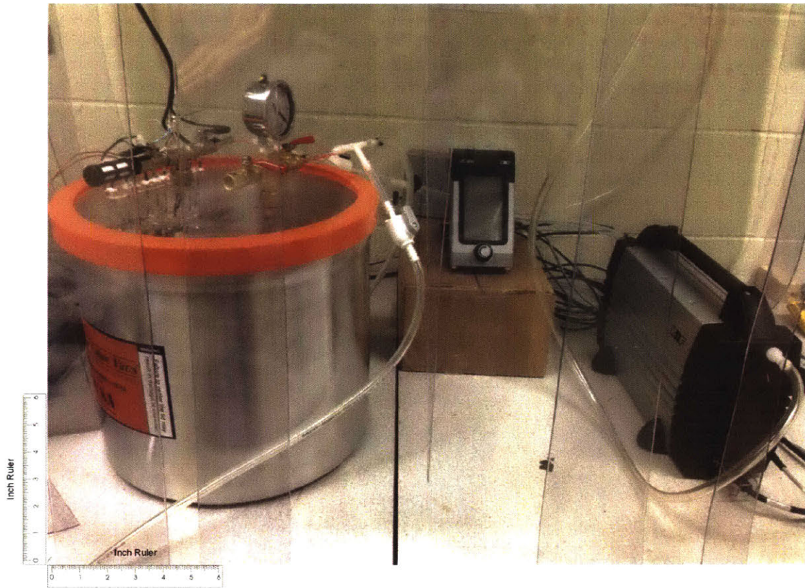
Figure 50: Sensors vacuum chamber setup with vacuum chamber, pump, and pump controller visible. An inch ruler is added for scale.
