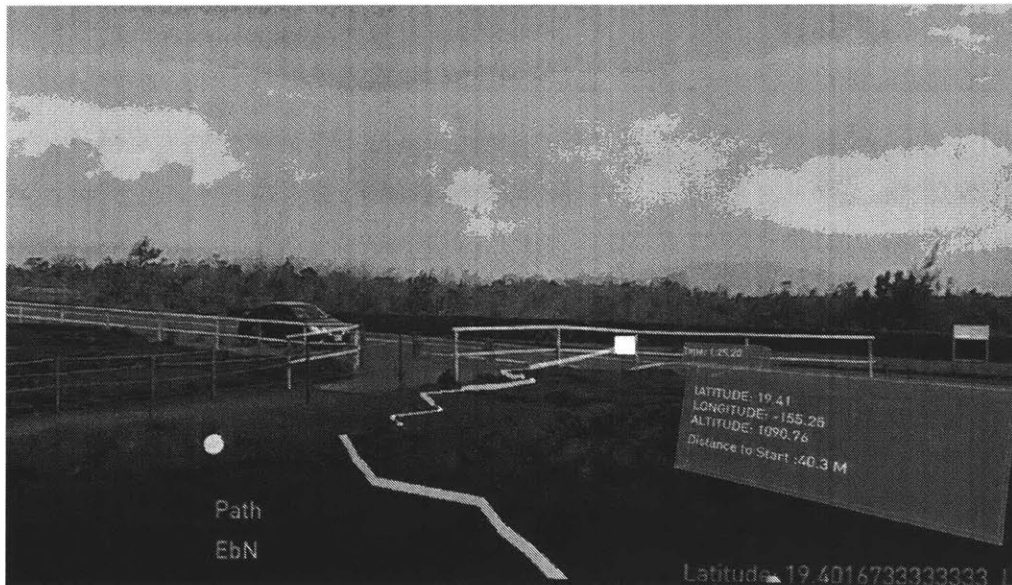
Figure 5-10: First person view of Holo-SEXTANT UI Includes path, waypoint, and status display
