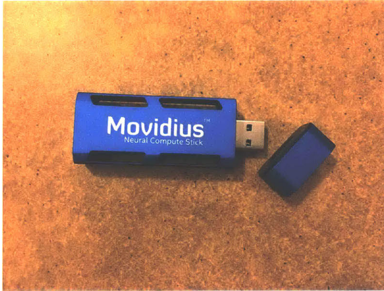
Figure 3-6: Intel Movidius Neural Compute Stick
