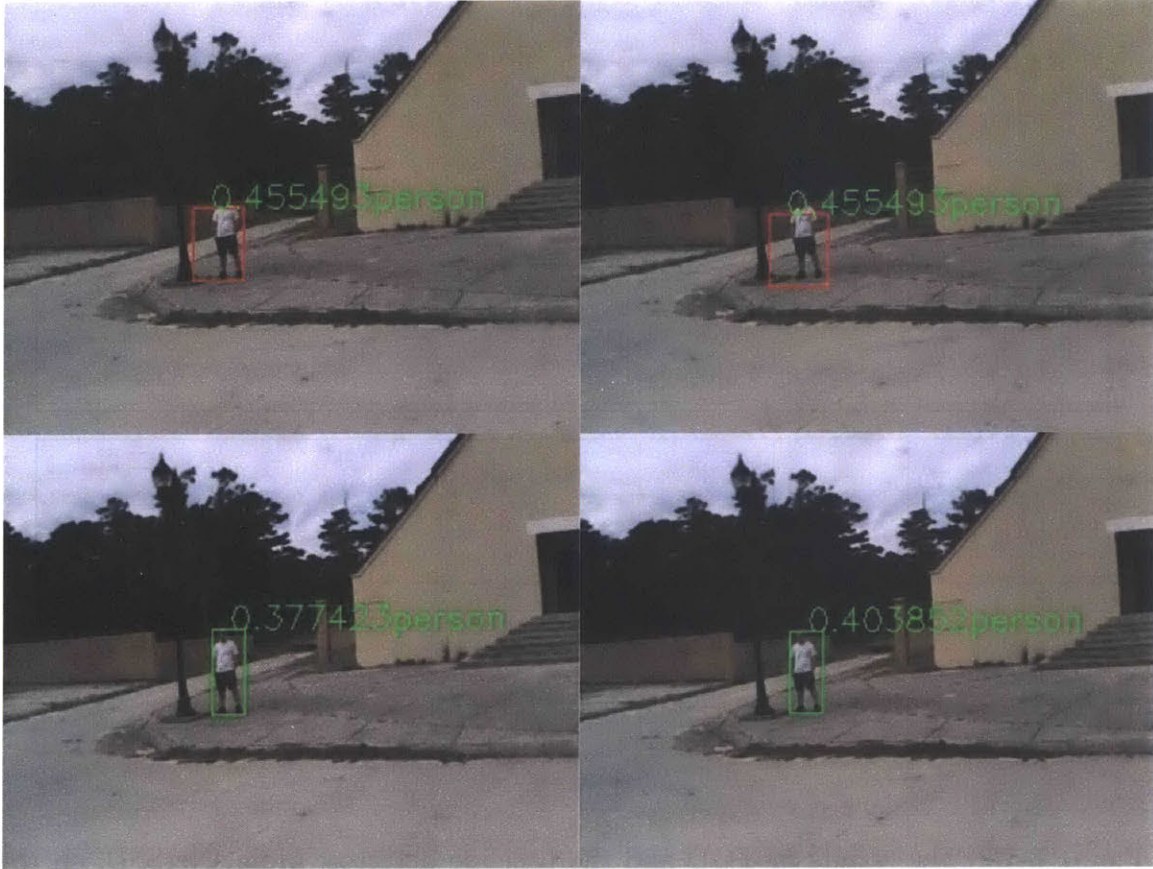
Figure 5-8: A poor result of TOD. The top row is from TOD running at a confidence threshold of 0.4 and the bottom row shows TOD running at a confidence threshold of 0.35. The red boxes are detections from the GOTURN tracker. The top row has poor detection results because of drift in the tracker from a bad target image. This does not occur in the bottom row because the detection output was not rejected by the threshold.
