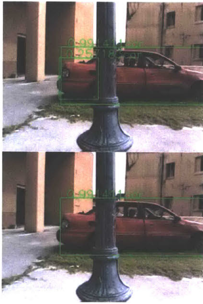
a) Example of the overlap non-maximum suppression step removing a false positive detection.
