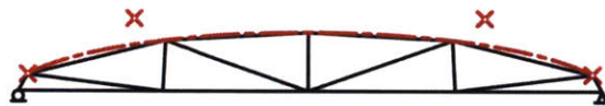
Figure 20: Creating the Grasshopper truss using a NURBS curve (shown in the dashed red line)
