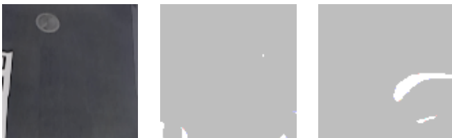
Fig. 5: Left: The cropped, re-sized and registered image. Middle: Example of a frame which contains no moving obstacle behind the corner. Right: Example of a frame which contains movement. The white areas correspond to a shadow signal.
