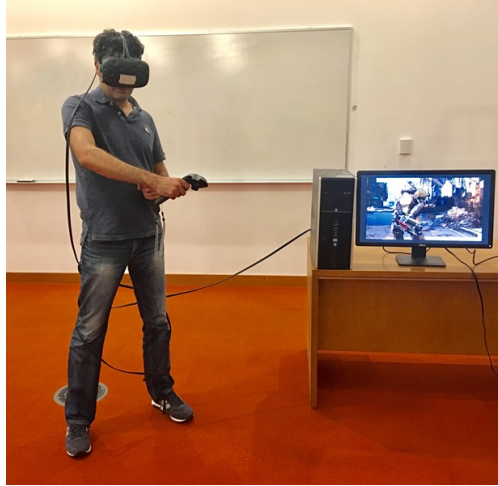
Figure 1-1: Virtual Reality experience: The headset's cable not only limits the player's mobility but also creates a tripping hazard.
