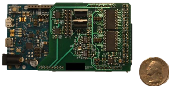
Figure 7-1: MoVR mirror’s controller board: The figure shows our custom-designed controller board for configuring the beam alignment and the amplifier gain in real time.
