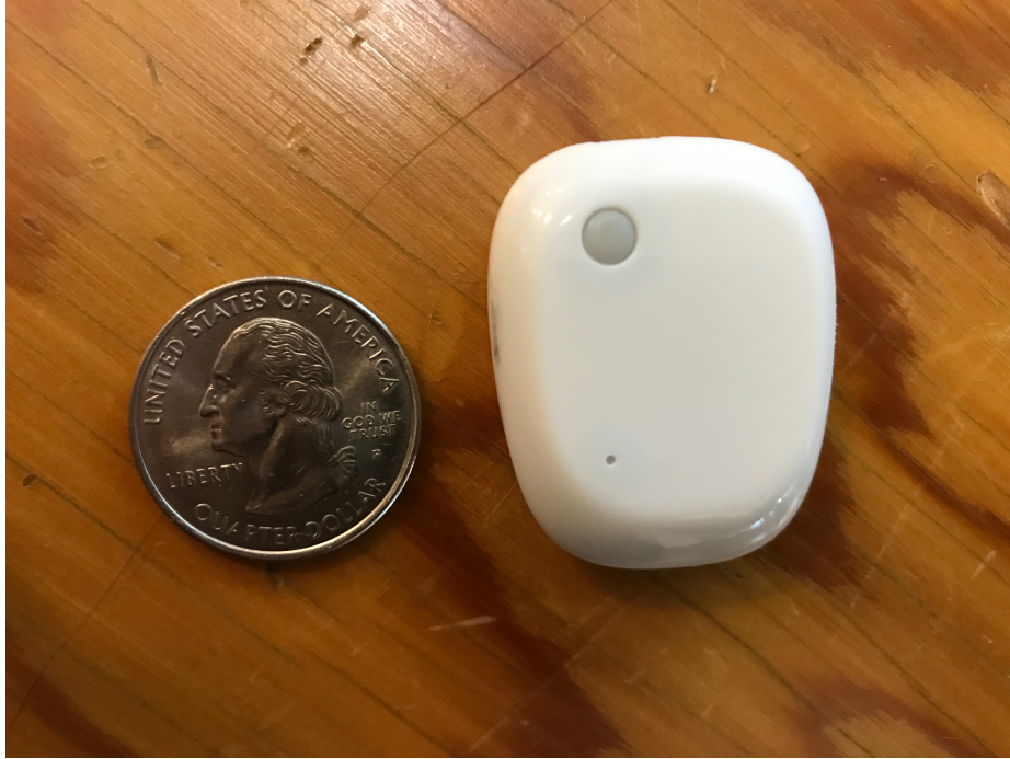
Figure 4-1: Metawear . The accelerometer sensor that we used. It is slightly bigger than a quarter. It can easily be carried in the pocket, on a clip on the belt or on a strap around the ankle.
