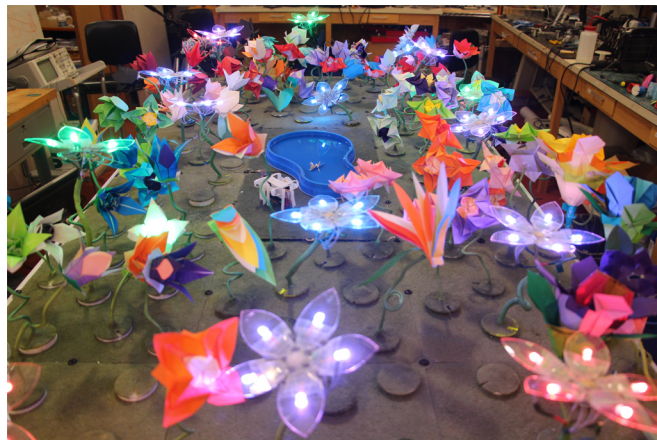
Fig. 1. The Robot Garden is a heterogeneous collection of distributed robots, including 100 actuated origami flowers and mobile foldable insects.
