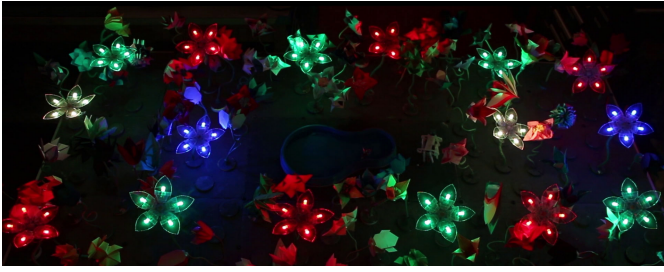
Fig. 11. A distributed greedy graph coloring algorithm finds an optimal 4-coloring of the robot garden (each tile is considered connected to its possibly 8 surrounding neighbors).
