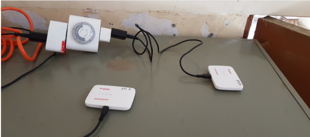
Figure 4-10: Picture of hotspot set up used to upload data to a remote server
