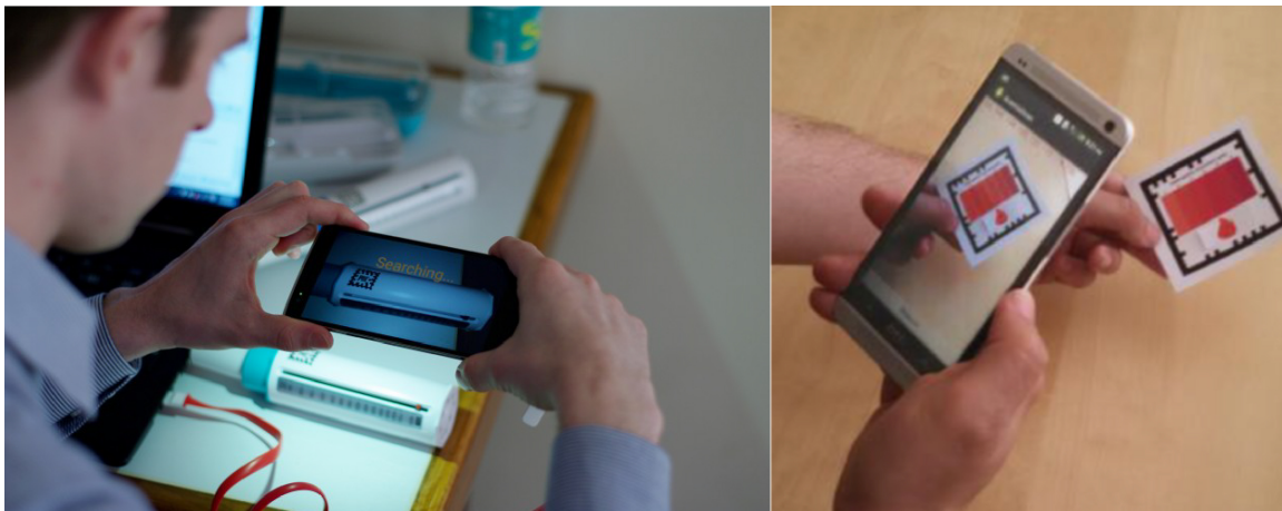
Figure 2-2: Examples of Prior Use of AR in our group — (left) AR App to automatically digitize the reading from a Peak Flow Meter; (right) a color test that uses AR to rectify the image and sample pixels from the correct colors
