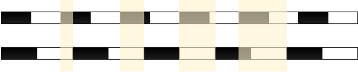
Figure 3-19: Phase shift discontinuity schematic
