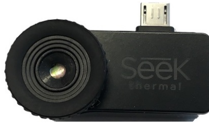
Figure 5-3: Thermal camera module used with thermal apps
