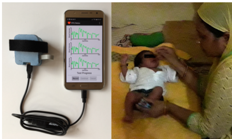
Figure 4-5: Photo of custom PPG device connected to Android phone (L). PPG device being applied to baby foot in a field study (R).
