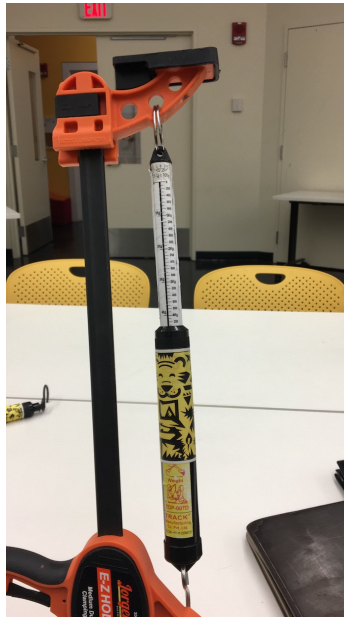
Figure 3-13: Scale Experiment Setup for Weight Measurement Validation
