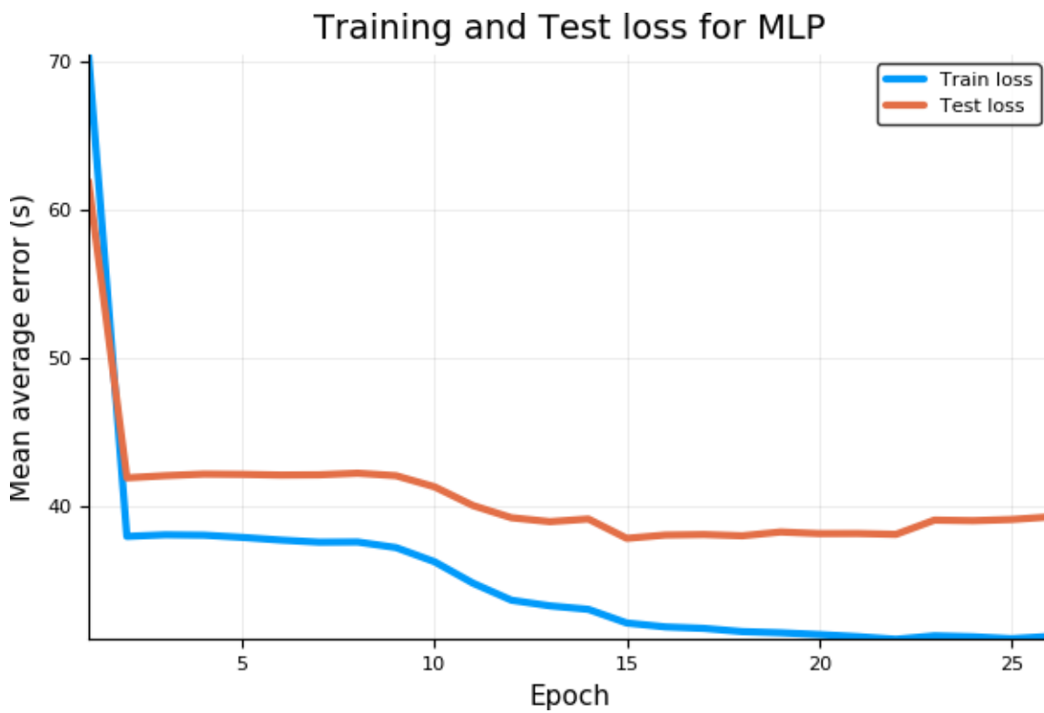
Figure 4-2: Loss for MLP model (lower is better). The MLP can capture more of the variation in outputs than the linear model.
