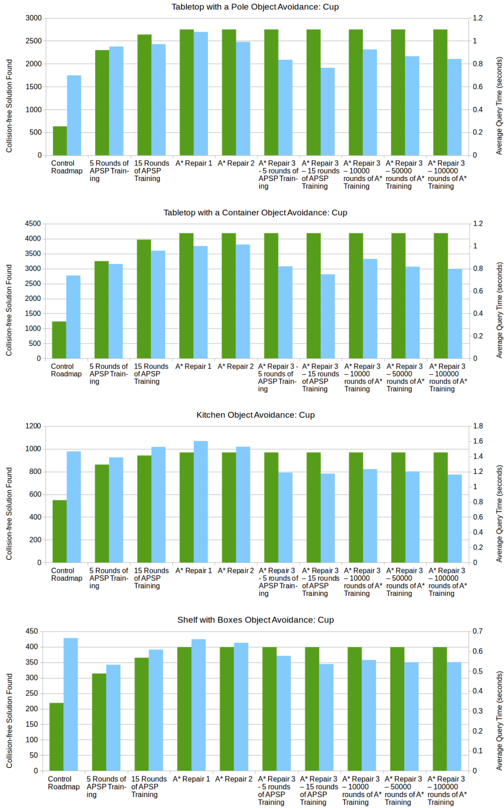
Figure A-16: Performance of solution caches developed with APSP Training in obstacle insertion experiment with Cup obstacle for all four environments
