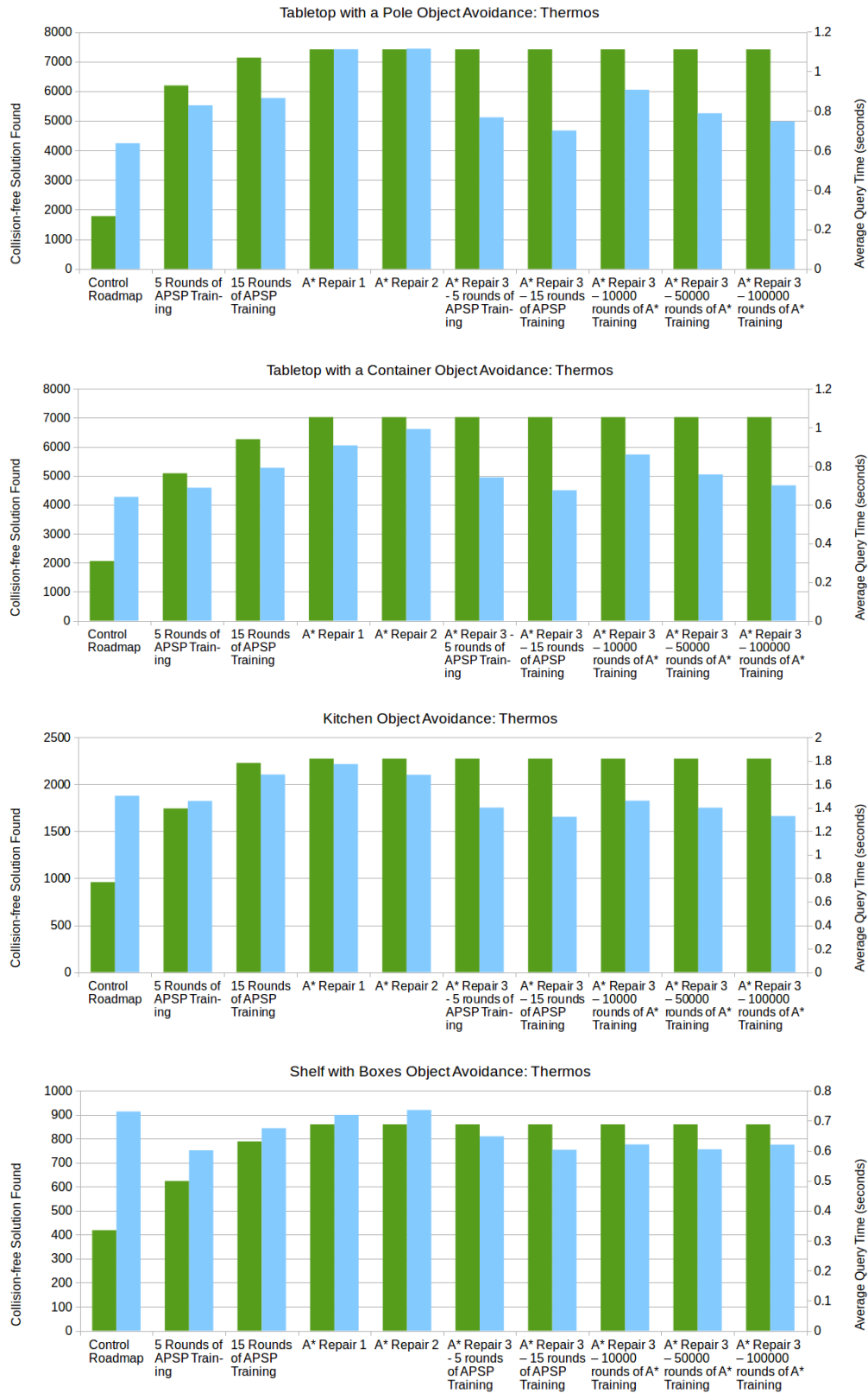
Figure A-17: Performance of solution caches developed with APSP Training in obstacle insertion experiment with Thermos obstacle for all four environments
