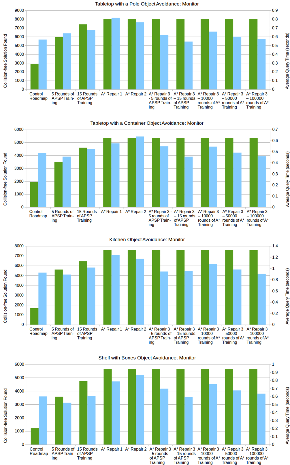
Figure A-18: Performance of solution caches developed with APSP Training in obstacle insertion experiment with Monitor obstacle for all four environments
