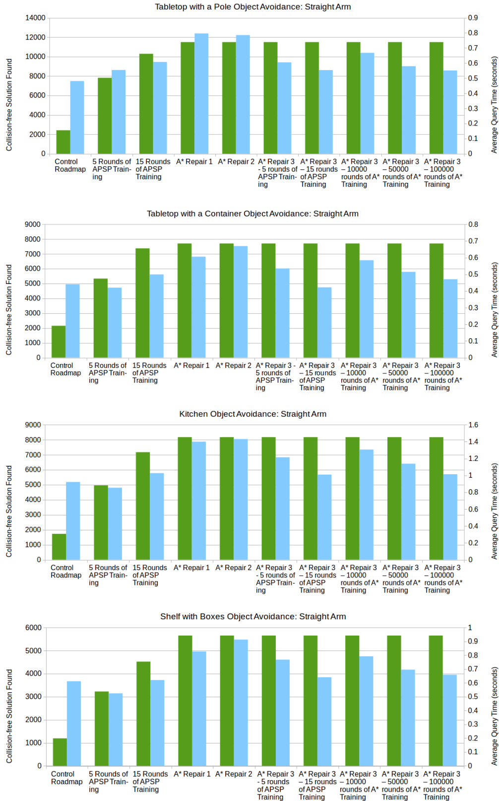
Figure A-20: Performance of solution caches developed with APSP Training in obstacle insertion experiment with Straight Arm obstacle for all four environments
