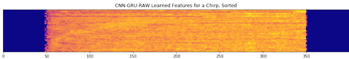
Figure 5-15: Learned features from the CNN-GRU-RAW for a 3 second chirp produced by Equation 5.1, where the rows are sorted according to their filter's most prominent frequency, as displayed in Figure 5-12. In the lower frequencies, you can make out a faint curve indicative of the log Mel filter banks in Figure 5-13.
