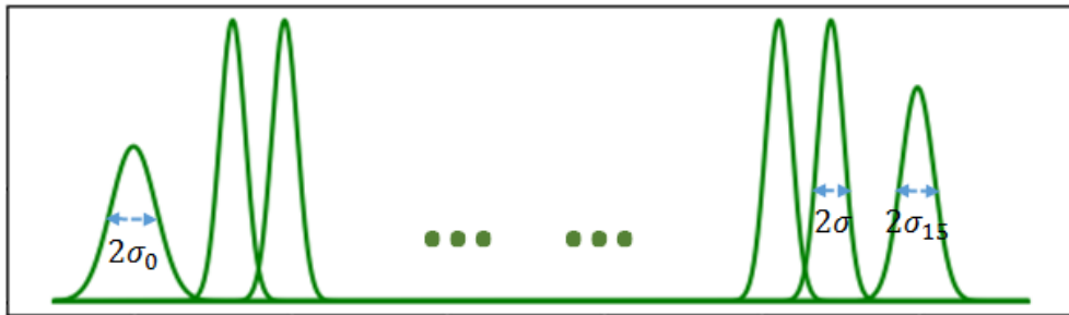
Figure 3-8: Flash channel model with 16-ary signal constellation. Note S_0 and S_{15} have higher variance. The separation between these two symbols and the other symbols is relatively high to balance out the raw error rate and maximize the channel capacity. The dots represent the rest of the 16 symbols with variance \sigma . Note the labels on the figure are twice the variance.
