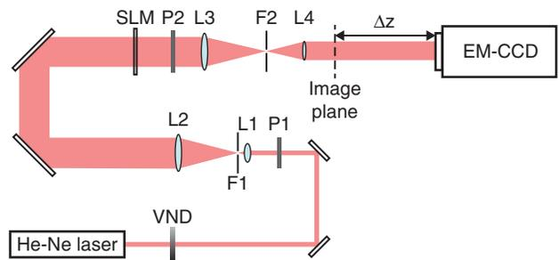
FIG. 1. Optical apparatus. VND, variable neutral density filter;  $P1$ – $P2$ , polarizers;  $L1$ ,  $10\times$ , 0.25 NA objective;  $L2$ , 100 mm lens;  $L3$ , 230 mm lens;  $L4$ , 100 mm lens;  $F1$ ,  $5 \mu\text{m}$  pinhole;  $F2$ , iris. SLM, transmissive spatial light modulator. Lenses  $L3$  and  $L4$  are confocal. The distance between the SLM and  $L3$  is 230 mm, the distance between  $L4$  and the image plane is 100 mm, and  $\Delta z = 400$  mm.
