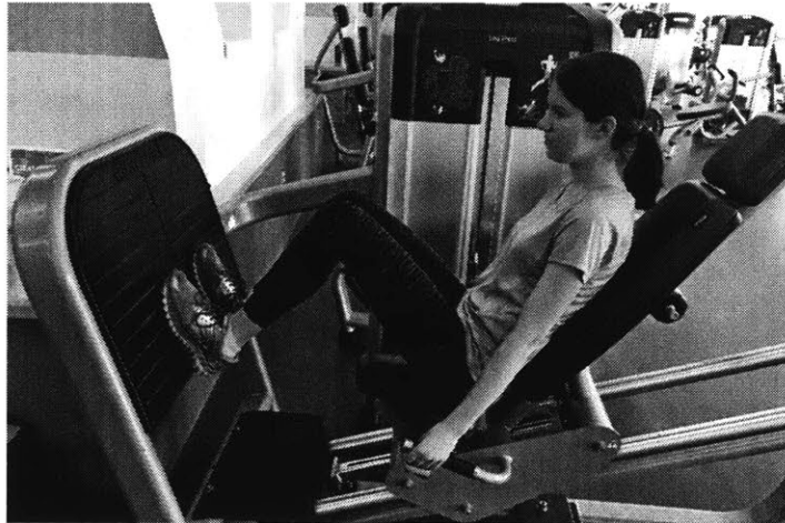
Figure 12: Experimental Setup on a leg press machine in the MIT Z Center. In this machine setup, the footplate was stationary, and chair was free to translate along an elevated ramp. An iPhone with accelerometer was placed on the moving weights inside the machine, and all athletes started the lifts from an initial inner leg angle of ~70 degrees.
