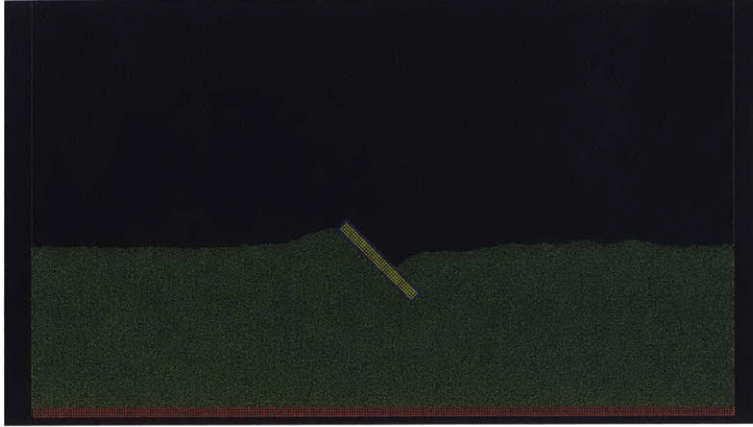
Figure 2-3: A output frame of the large wheel from the 'Trudging' Case. Note that it sinks substantially deeper into the granular material than the walking case, and displaces substantially more grains.
