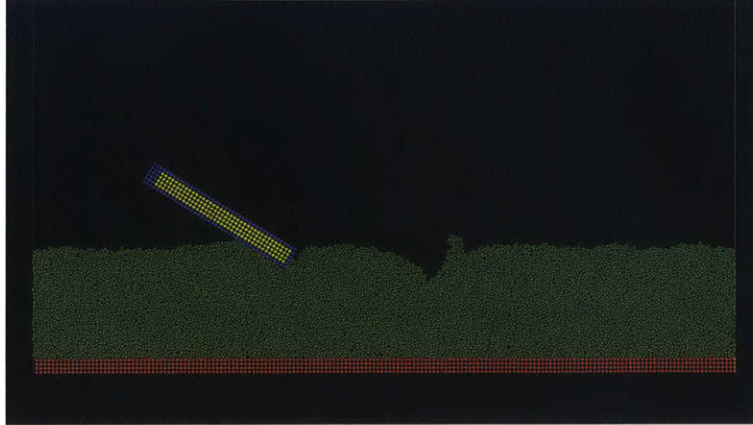
Figure 2-5: An output frame from the big wheel simulation from the muddy case. Note that the new potential between grains allows for the sand to create otherwise impossible formations.
