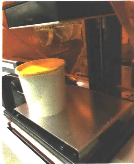
Figure 7: Dip-coating set-up. An aluminum sheet is fitted to the top of the resin tank of the Form 1+ printer so that the dip-coating container of Plasti Dip® can sit securely.
