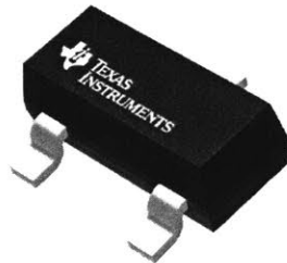
Figure 3.1: Linear Hall-Effect Sensor from Texas Instruments. These Hall-effect sensors are available in four different varieties with different sensitivities and data ranges. Image courtesy of Texas Instruments.
