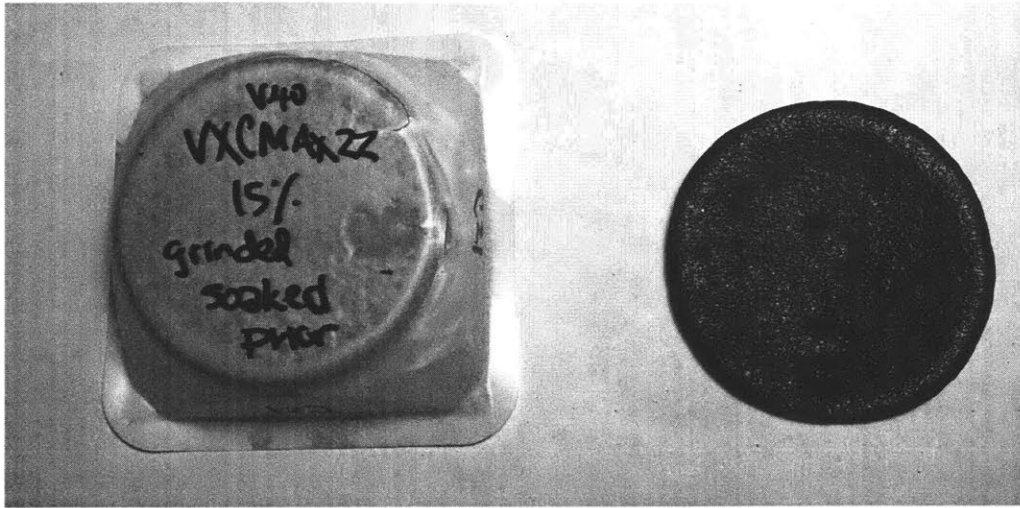
Figure 2.1: Typical Piezoresistive Material Test Sample. Different variations of polyurethane and silicone thermosets were combined with several different conductive particulates. Here, Vytaflex 40 was combined with specialty carbon black at 15 percent total mass. The resulting samples were then judged for quality of cure and piezoresistive properties.
