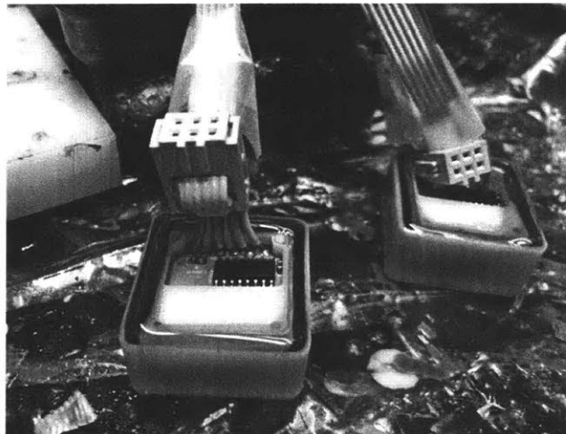
Figure 3.9: Hall-Effect Sensor PCB Elastomer Mold. The sensor PCB and back-piece are placed in the Vytaflex 20 matrix and allowed to fully cure.
