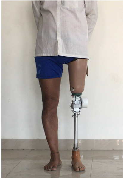
FIGURE 5. Subject wearing the knee prosthesis with the damper prototype. The knee prosthesis was attached to the socket, which interfaces with the residual limb and the pylon, which interfaces with the prosthetic foot.
